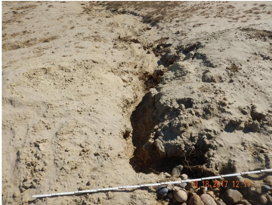
Photo 14: Closer look at blowout seen in previous photos. 6 foot measuring stick for reference.
