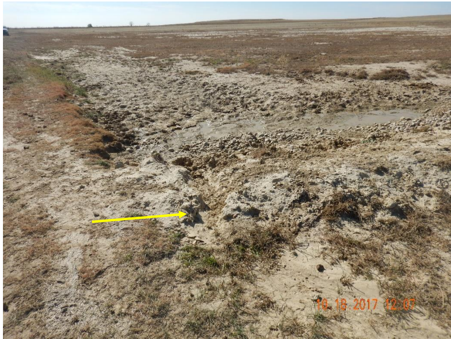
Photo 6: Photo taken from the east end of the location, facing southwest. Continued from photo 5. Photo shows area of the BMP that has been eroded out.
