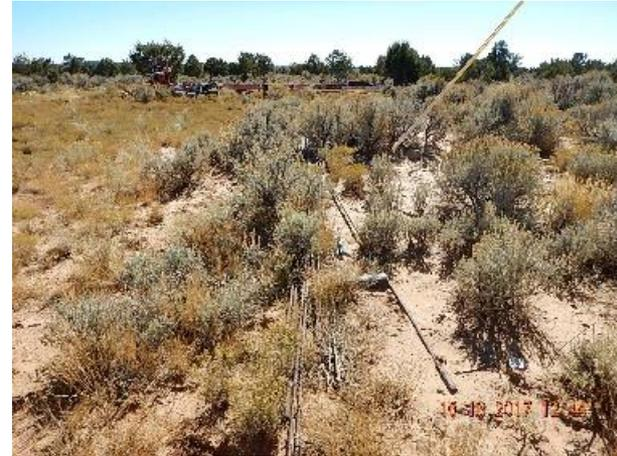
**Photo 8: Sucker rods and valve at edge of location.**
