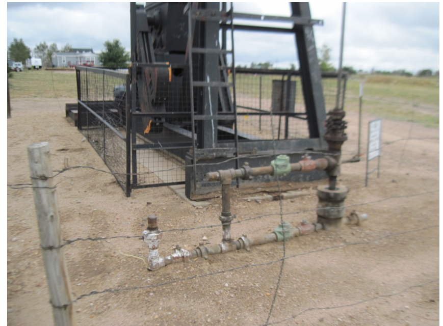
NEED BRADENHEAD PLUMBED TIO SURFACE
