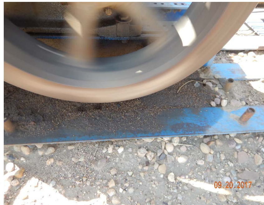
Photo #4 - Localized, oil-stained soil beneath prime mover.
