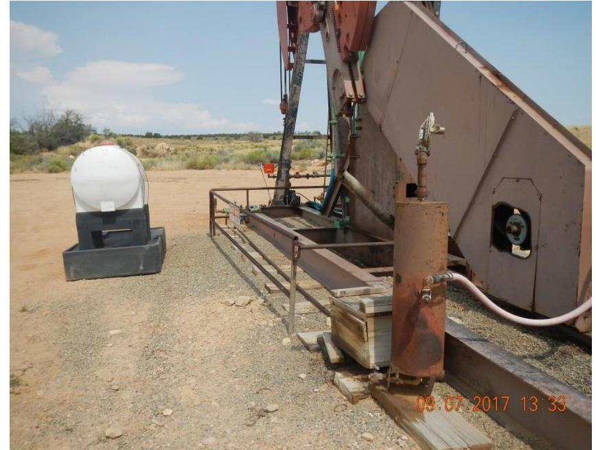
Unused chemical injection system.
