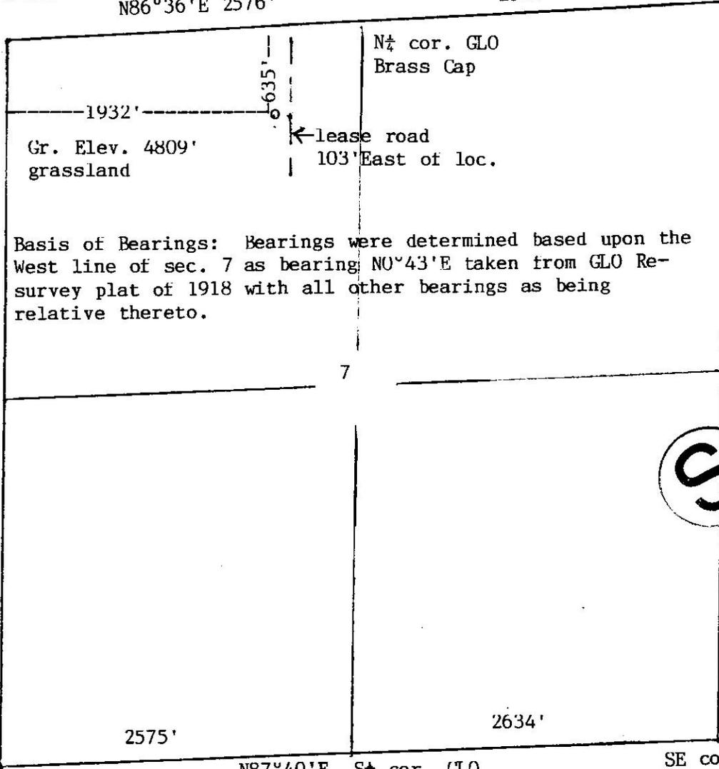
Basis of Bearings: Bearings were determined based upon the West line of sec. 7 as bearing N0°43'E taken from GLO Re-survey plat of 1918 with all other bearings as being relative thereto.
