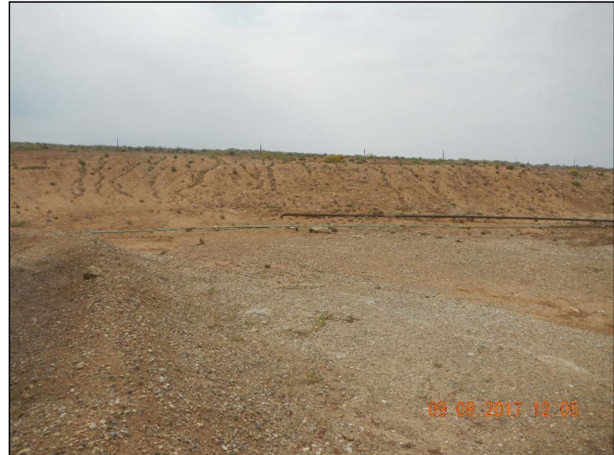
Photo 6. Erosion rills coming onto location.
