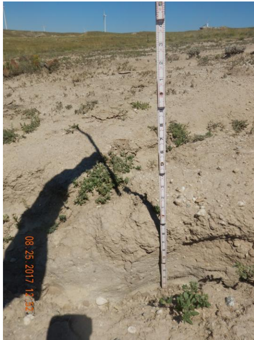
Photo 38: Photo taken from the southwest of the pit. Photo shows gulley erosion due to stormwater runoff from the location. Gulley seen here is ~1.5 feet in depth.
