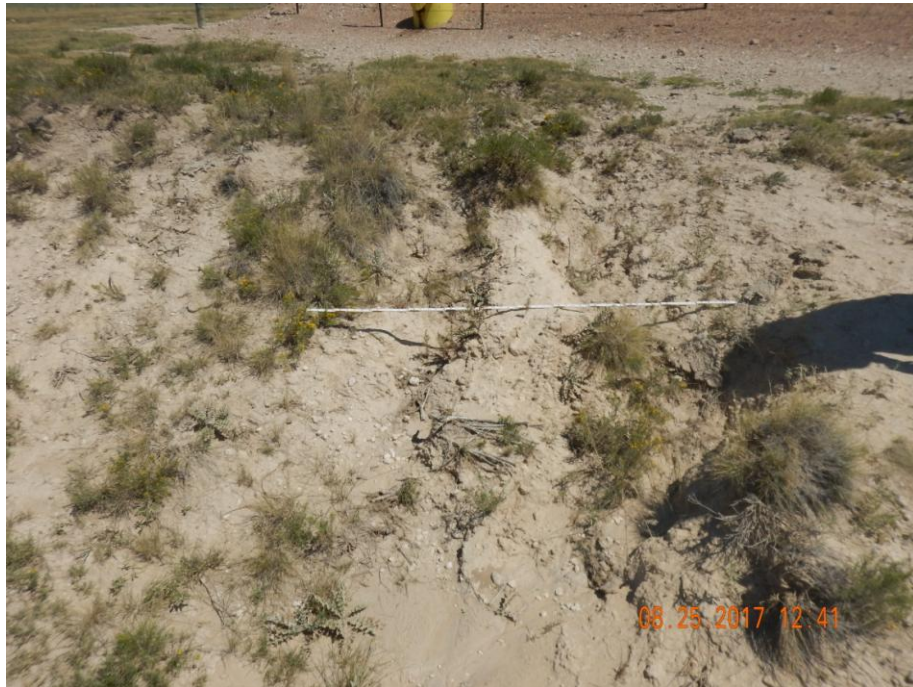
Photo 8: Photo taken on the northern part of the location, just west of the tank battery. Photo shows degradation to the location due to stormwater erosion. Erosion will need to be repaired and stabilized. Required BMPs will need to be installed and maintained in accordance to 1002.f to prevent further degradation. 6 foot measuring stick for reference.
