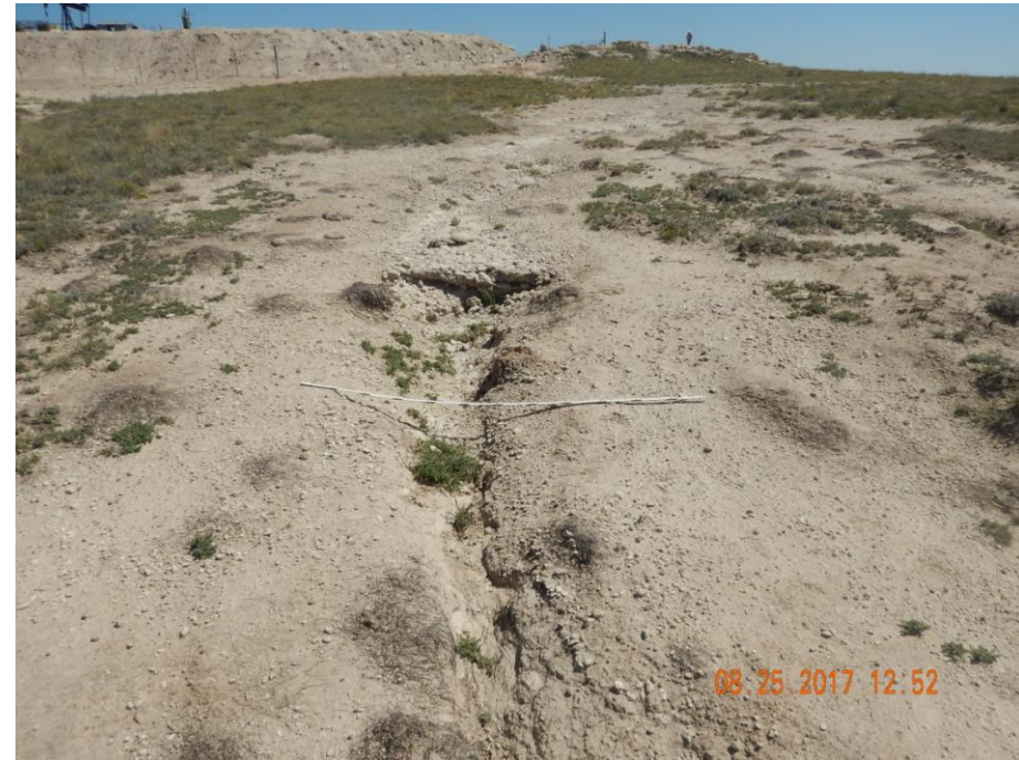
Photo 39: Photo taken from the southwest of the pit, facing east. Photo shows stormwater runoff from the location has caused erosion degradation on the adjacent lands. Erosion will need to be repaired and stabilized. Required BMPs will need to be installed and maintained in accordance to 1002.f to prevent further degradation. These areas will need to be re-vegetated/reclaimed. Soil testing is advised as contaminants may exist preventing vegetation from re-establishing.
