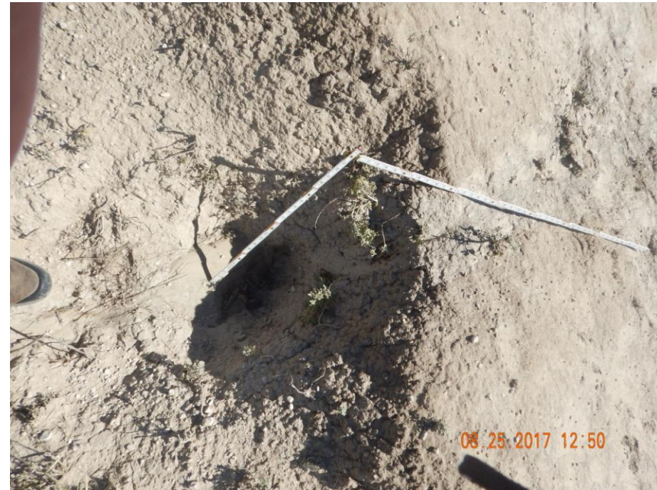
Photo 31: Photo taken from the west of the pit. Photo shows large headcuts have formed due to stormwater erosion from the location. Headcut seen here is ~2 feet in height. There are other headcuts in the area that appear to be larger in size.
