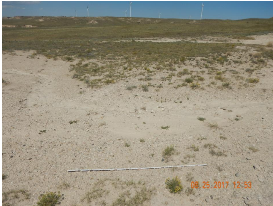
Photo 42: Photo taken from the southwest end of the pit, facing north. Photo shows stormwater runoff from the location has caused erosion degradation on the adjacent lands. Erosion will need to be repaired and stabilized. Required BMPs will need to be installed and maintained in accordance to 1002.f to prevent further degradation. These areas will need to be re-vegetated/reclaimed. Soil testing is advised as contaminants may exist preventing vegetation from re-establishing. 6 foot measuring stick for reference.
