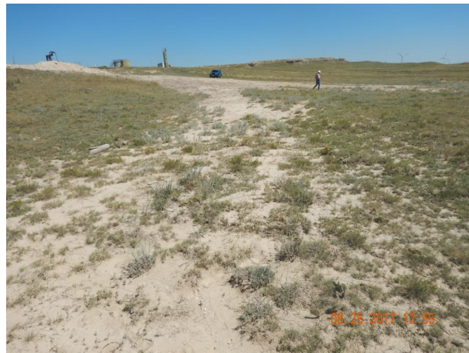
Photo 47: Photo taken from the south and west end of the pit, facing northeast. Photo shows stormwater runoff from the location has caused erosion degradation on the adjacent lands. Erosion will need to be repaired and stabilized. Required BMPs will need to be installed and maintained in accordance to 1002.f to prevent further degradation. These areas will need to be re-vegetated/reclaimed. Soil testing is advised as contaminants may exist preventing vegetation from re-establishing.
