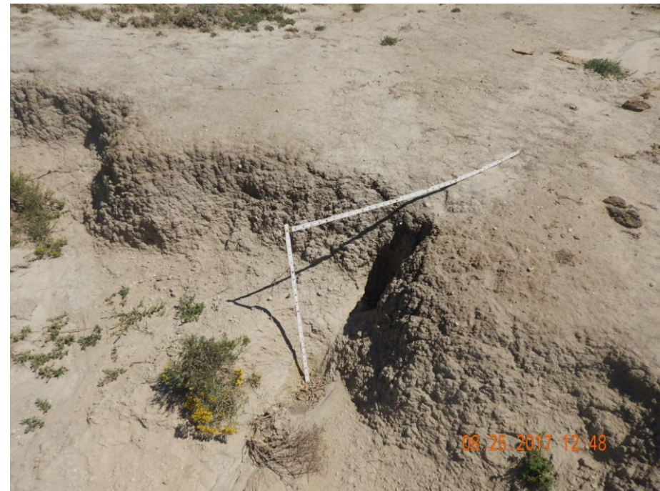
Photo 27: Photo taken from the degraded areas west of the pit. Photo shows large headcuts have formed due to stormwater erosion from the location. Headcut seen here is ~2 feet in height. There are other headcuts in the area that appear to be larger in size.
