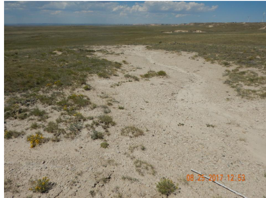
Photo 43: Photo taken from the southwest end of the pit, facing west. Photo shows stormwater runoff from the location has caused erosion degradation on the adjacent lands. Erosion will need to be repaired and stabilized. Required BMPs will need to be installed and maintained in accordance to 1002.f to prevent further degradation. These areas will need to be re-vegetated/reclaimed. Soil testing is advised as contaminants may exist preventing vegetation from re-establishing. 6 foot measuring stick for reference.
