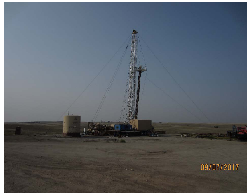
Photo #2 – Workover rig on-site on date of inspection.
