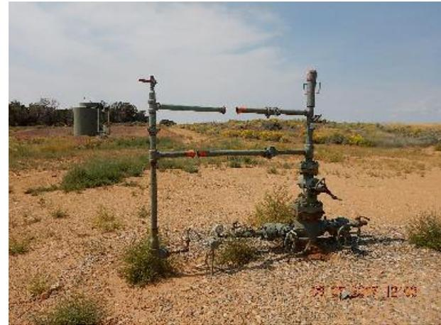
Photo 2: Disconnected wellhead and riser.
