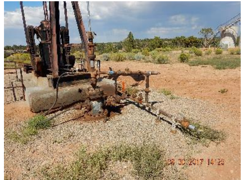
Photo 2: Wellhead with impacted soil around base of wellhead and 1" steel riser.
