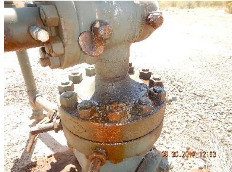
Photo 4: Leak at wellhead.
