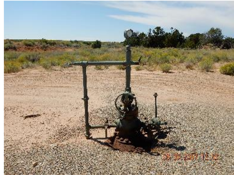
Photo 2: Disconnected wellhead and riser.
