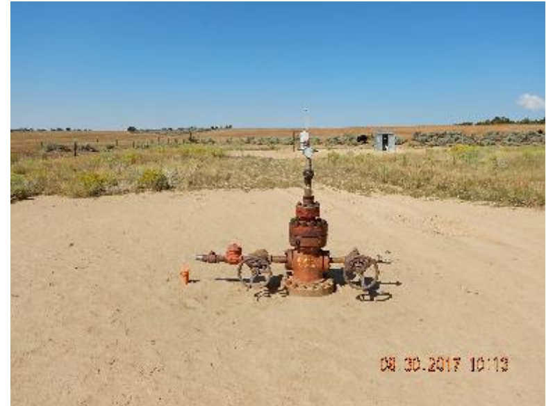
Photo 2: Disconnected wellhead and flowline riser.
