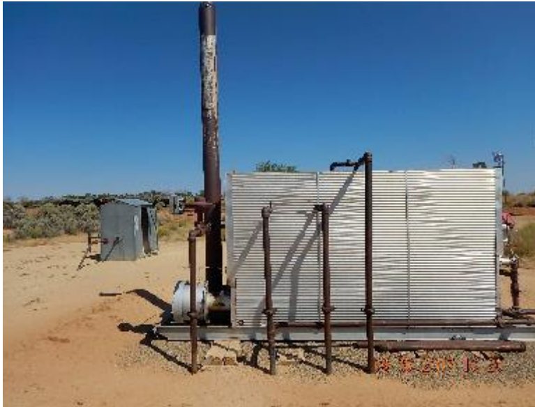
Photo 5: Separator and risers.
