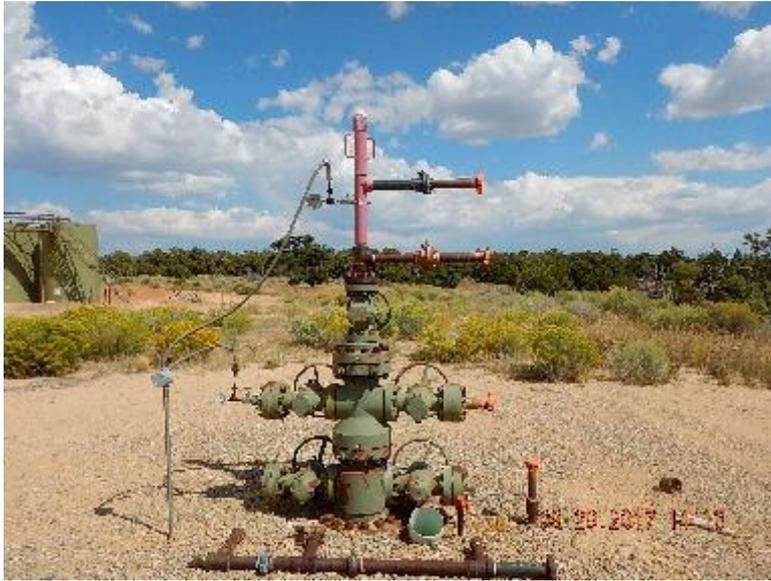
**Photo 3: Wellhead with production tree removed. Riser painted orange.**
