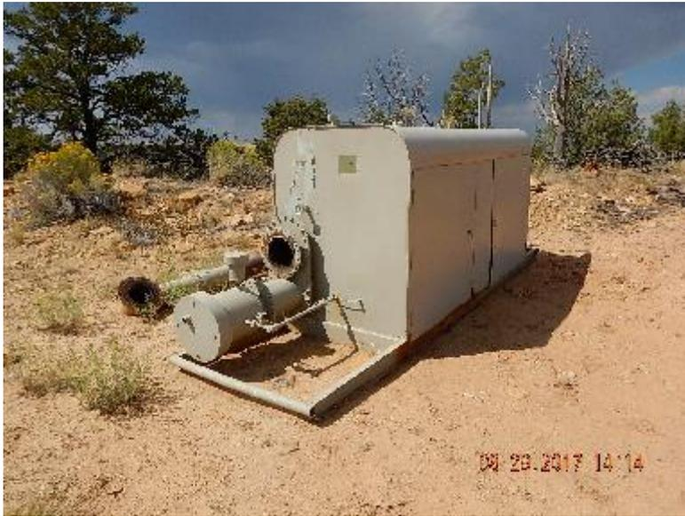
**Photo 5: Disconnected separator and stack in NW corner of location.**
