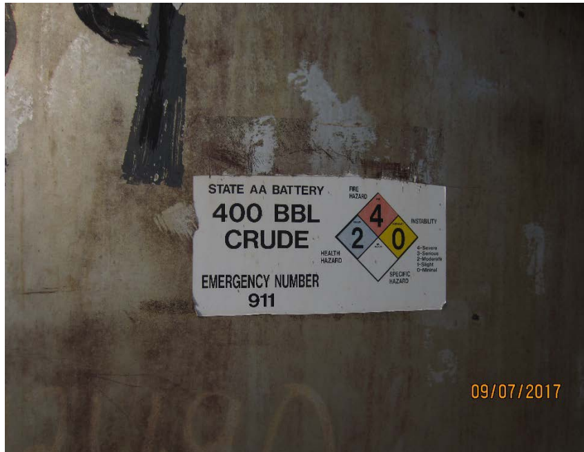
Photo #3 – Label and placard on crude oil AST.
