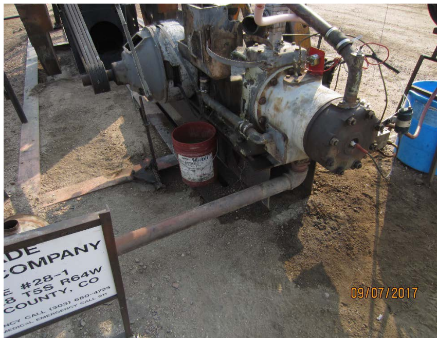
Photo #3 – Localized, oil-stained soil beneath prime mover.
