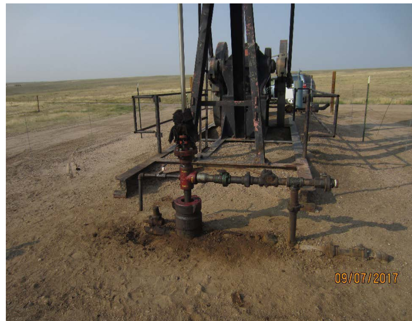
Photo #4 – Localized, oil-stained soil at wellhead. Note oily rag tied above stuffing box.
