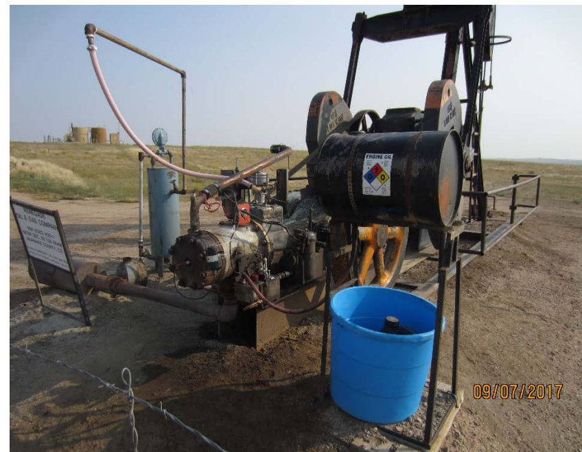
Photo #2 – Localized, stained soil beneath day tank and prime mover.
