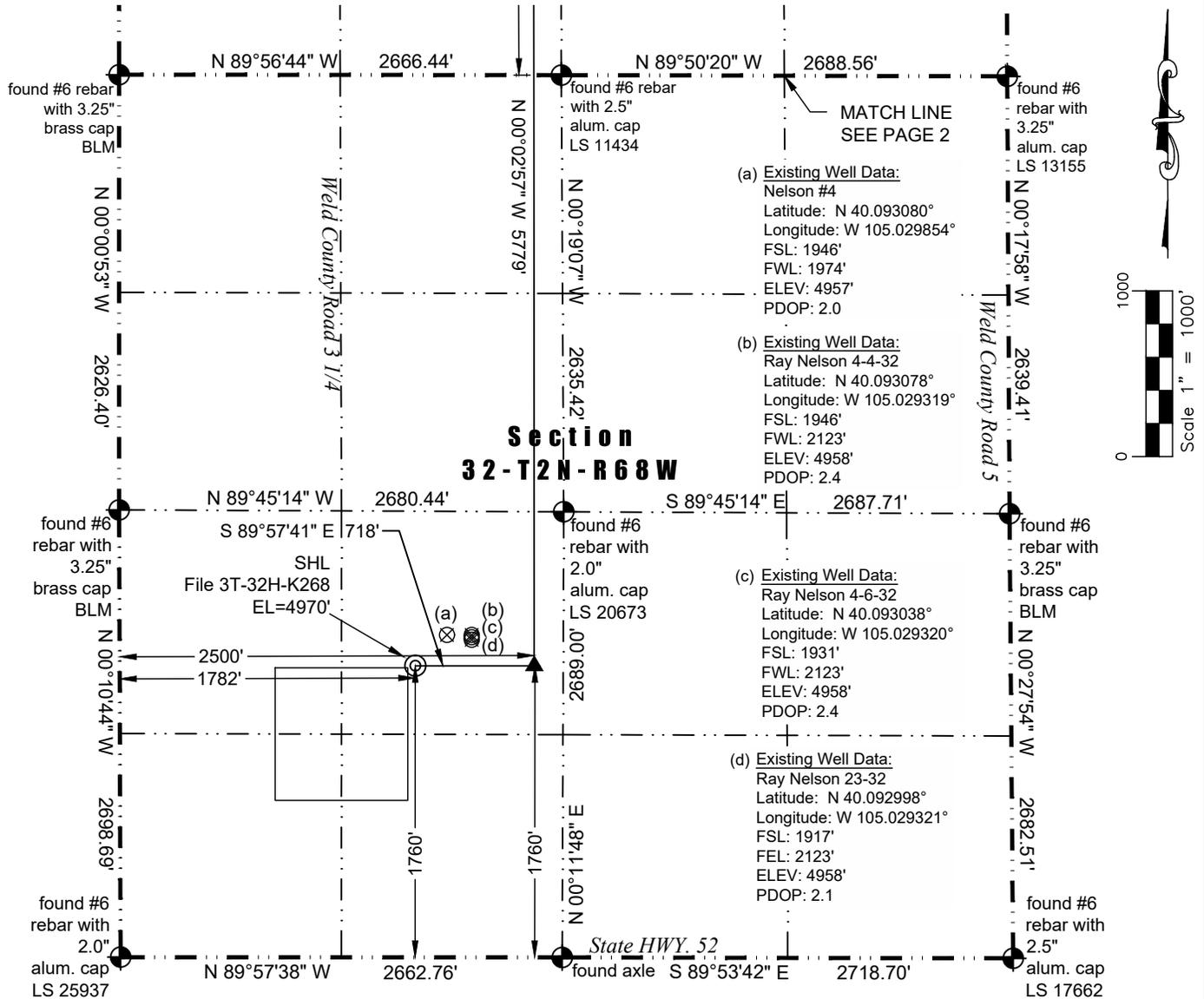
In accordance with a request from Jay Knutson of Crestone Peak Resources, Washburn Land Surveying, LLC has determined the location of the **File 3T-32H-K268** well site to be SHL: 1760' FSL and 1782' FWL, (TPZ: 1760' FSL and 2500' FWL), (BHL: 2215' FSL and 2500' FWL), as measured at ninety (90) degrees from the section lines of Sections 20 and 29, Township 2 North, Range 68 West of the 6th Principal Meridian, Weld County Colorado.
