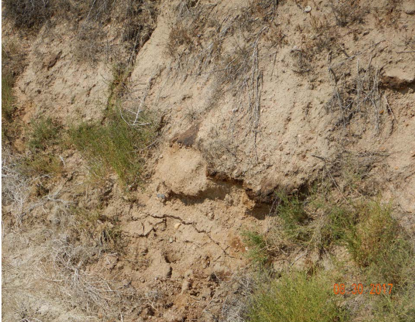
Photo #19 – Localized, oil-stained soil at NE corner of pit.
