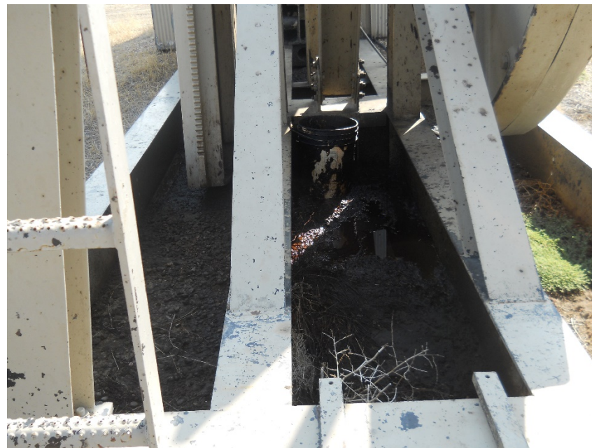
Front of pump jack skid looking east. North side and center of skid have stained soil and standing fluid, 5 gallon open top container with no wildlife protection
