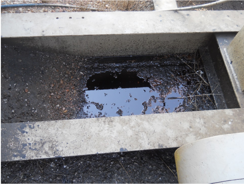
Stained soil in skid of pump jack, north side. Standing fluid appears to be used motor oil.
