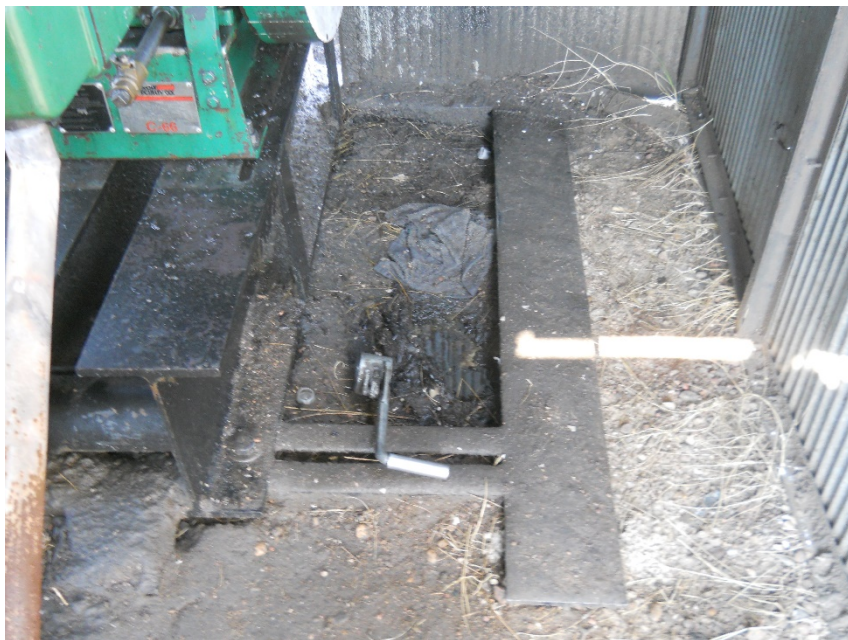
Stained soil under pump jack motor on north side, standing fluid appears to be used motor oil
