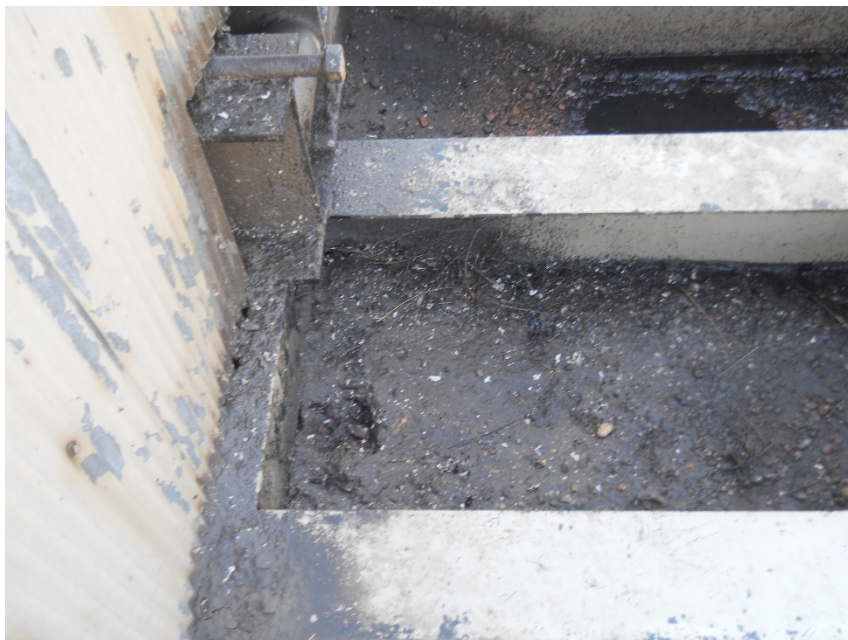
Stained soil in skid of pump jack on north side and middle. Standing fluid appears to be used motor oil leaking from pump jack motor
