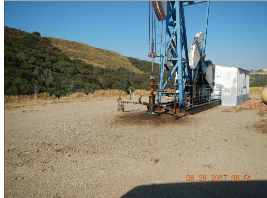
Photo 2. Stained soil at wellhead.
