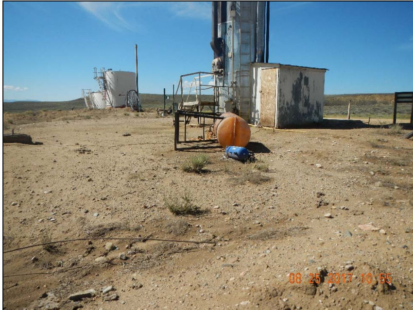
Photo 1. Methanol container knocked over with no secondary containment.
