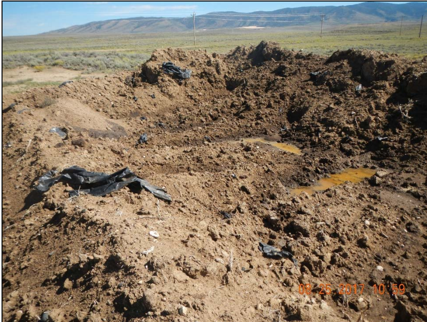
Photo 3. Land farm area with no containment. Berm around perimeter is unconsolidated and contains pieces of debris.
