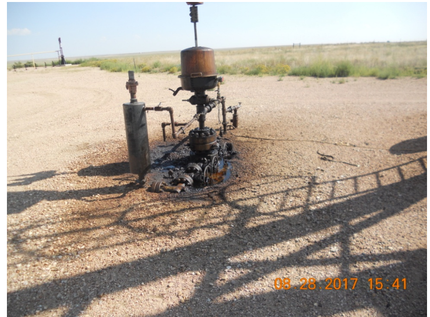
Photo 2. Stained soil at production tank leaking load line
