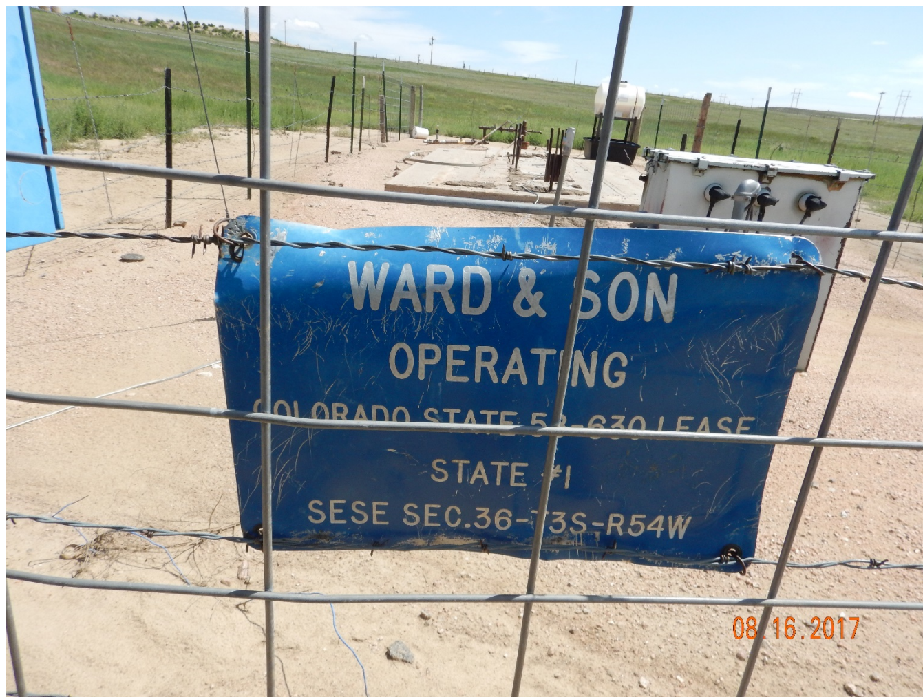
Figure 1 - Well sign lacking operator emergency contact information.
