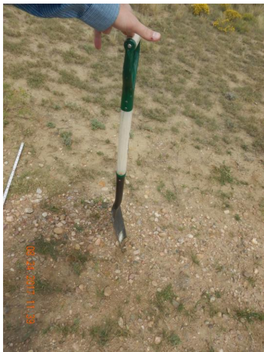
Photo 7: Photo taken from the access road. Photo shows gravel/road base remaining on location. Inspector had attempted to dig a soil pit to test access road for compaction. Inspector was unable to penetrate the soil more than a few inches; compaction alleviation has not been performed.
