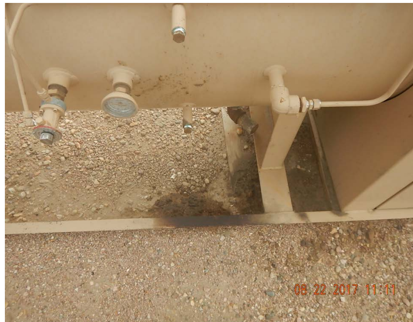
Photo 1: Stained soil outside of separator
