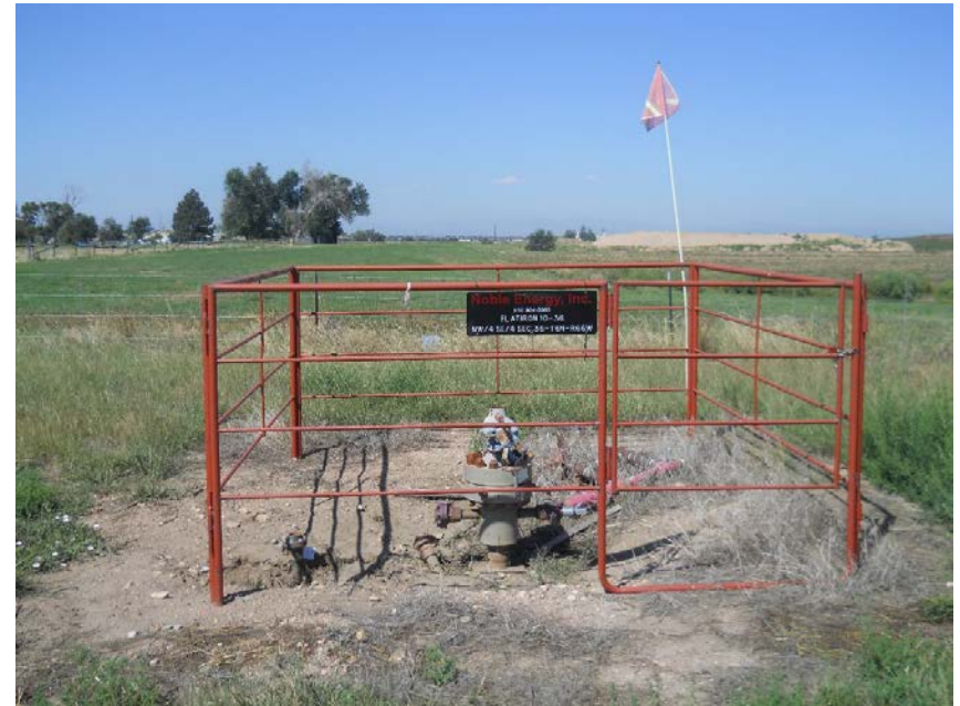
Wellhead looking west. Well is TA, no MIT records
