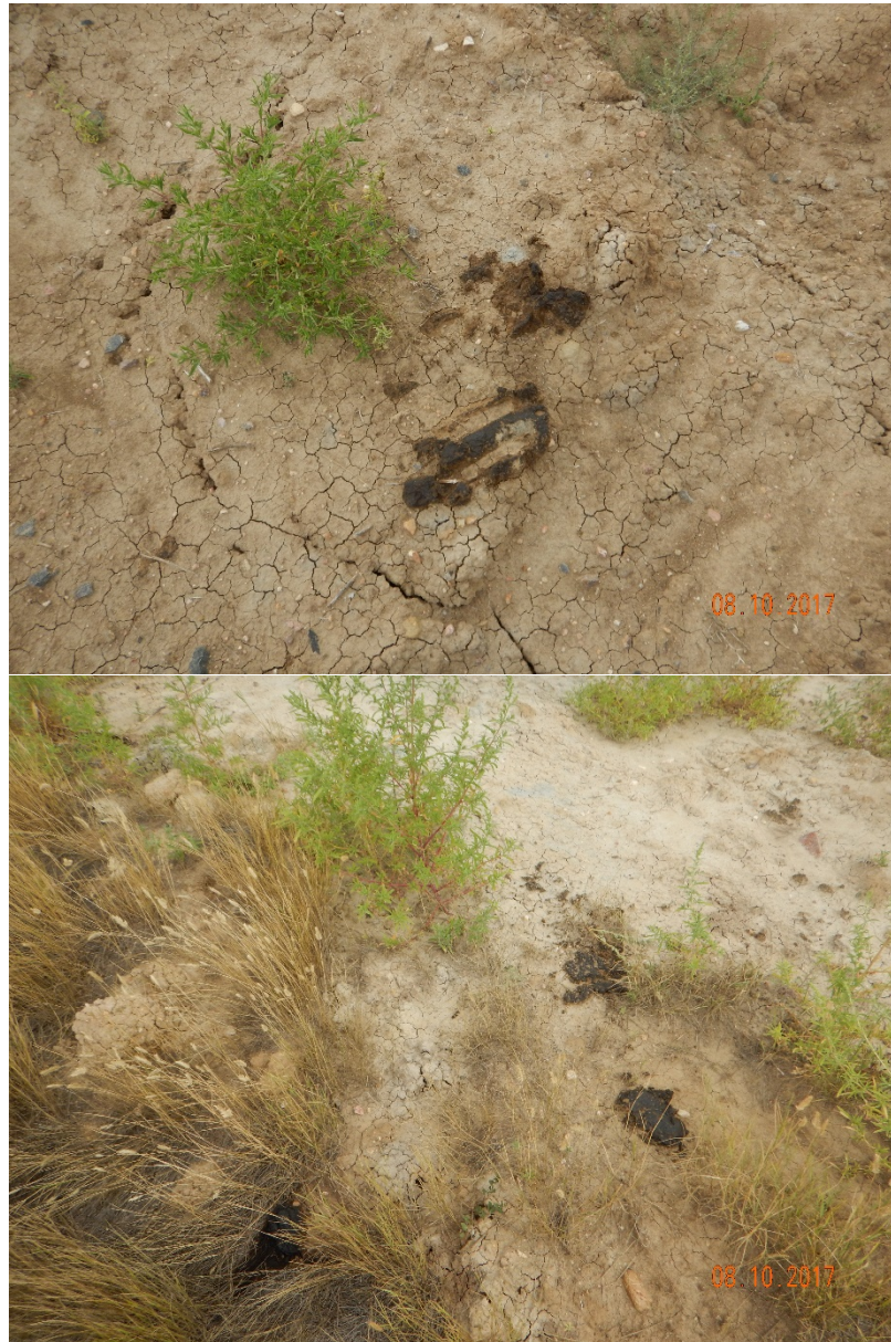
Figure 4 - Localized, oil-stained soil and apparent drilling mud on east side of former excavation.
