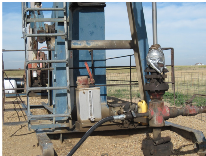
WELLHEAD CHEMICAL POT AND HIGH PRESSURE DUCT TAPE AND RAGS
