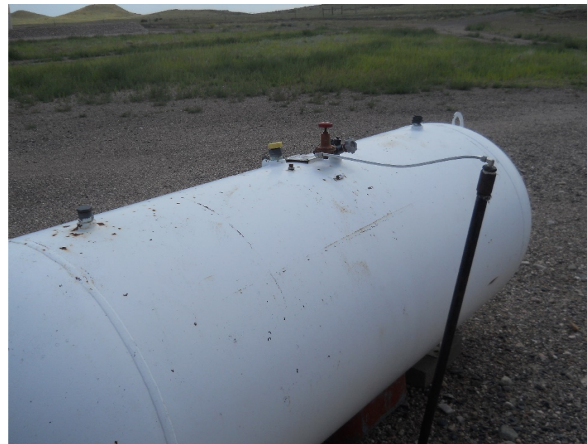
Propane tank on east side of pump jack with no labeling
