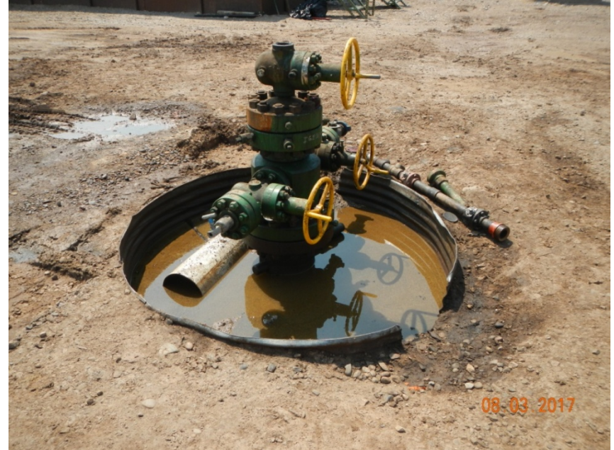
Photo 4: View of what appears to be oil and water in wellhead cellar.
