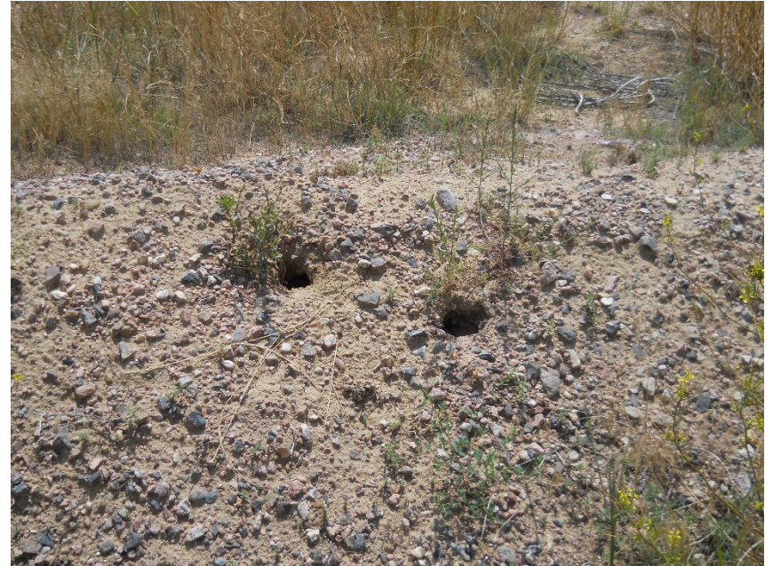
Animal burrow in northeast side of tank berm
