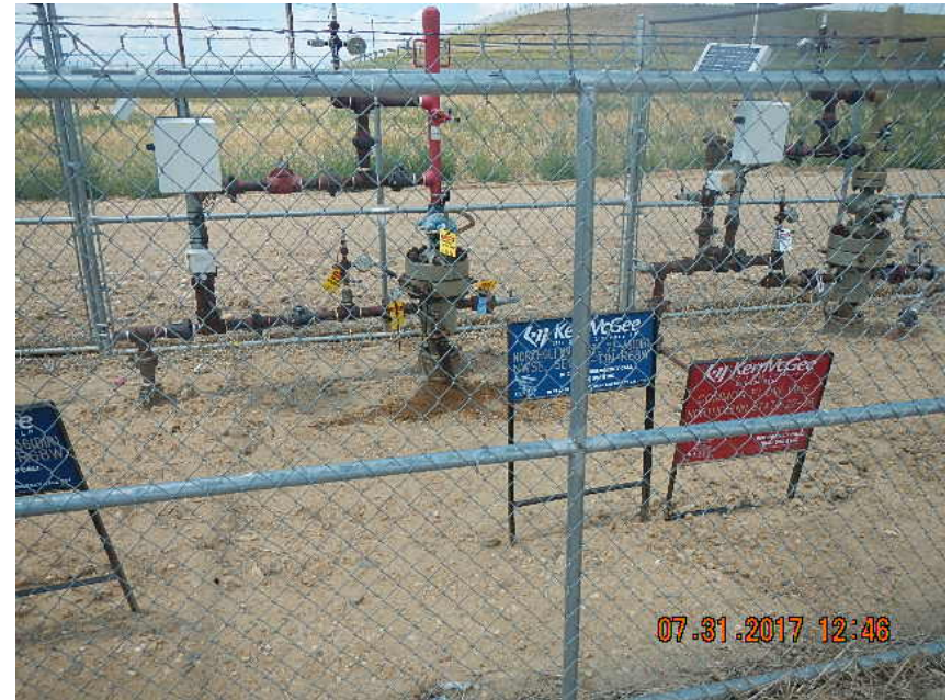
STAINED SOIL AT WELLHEAD
