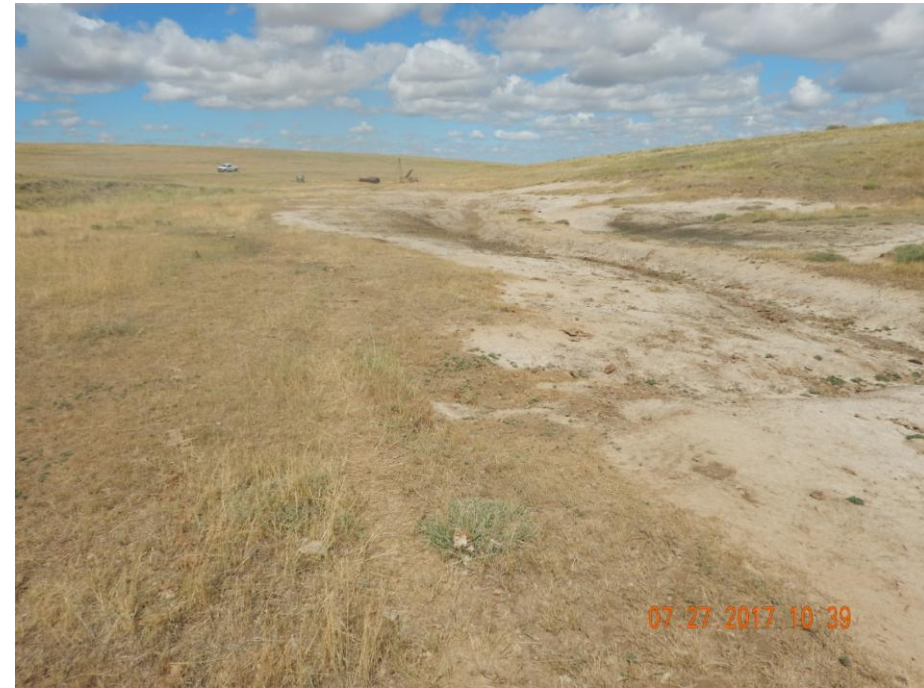
Photo 2: Photo taken from the south side of the drainage, adjacent to the pit and well location, facing northwest. Photo shows area of degradation that remain un-stabilized. Further degradation since previous inspection evident. See photos from inspection doc. # 682500927 for additional details.
