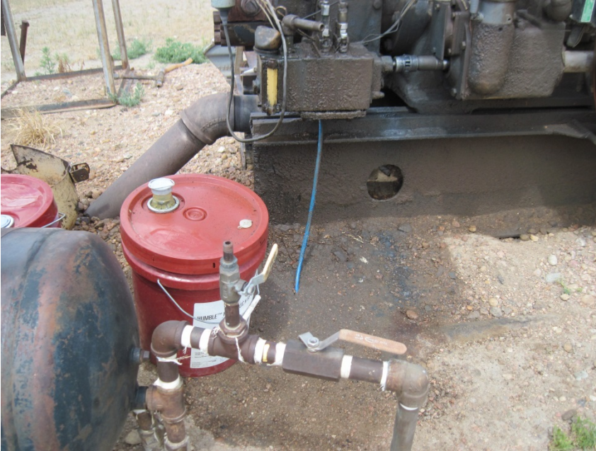
Stained soil at motor mounts
