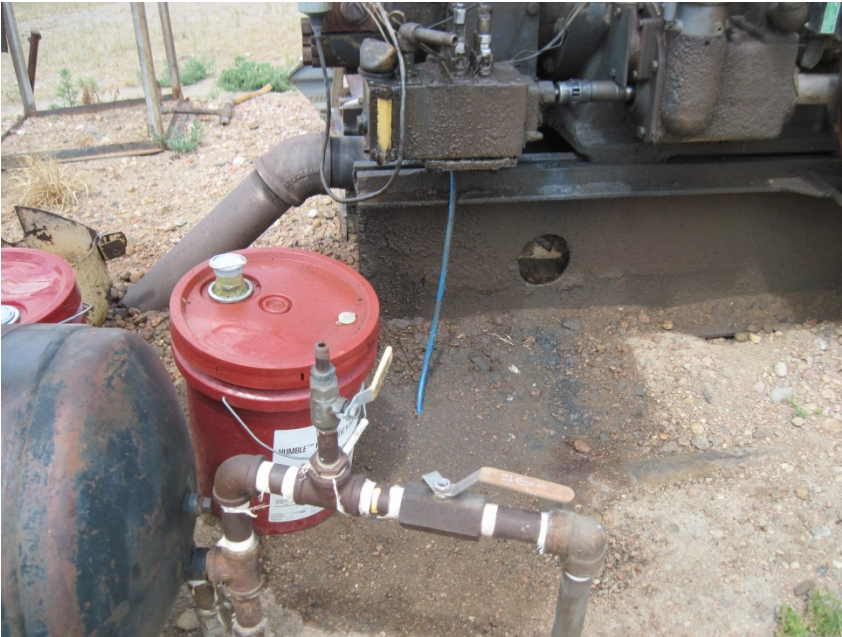
Stained soil at motor mounts
