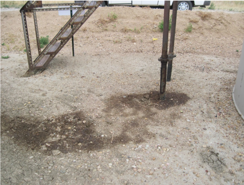
Stained soil inside berms at tank
