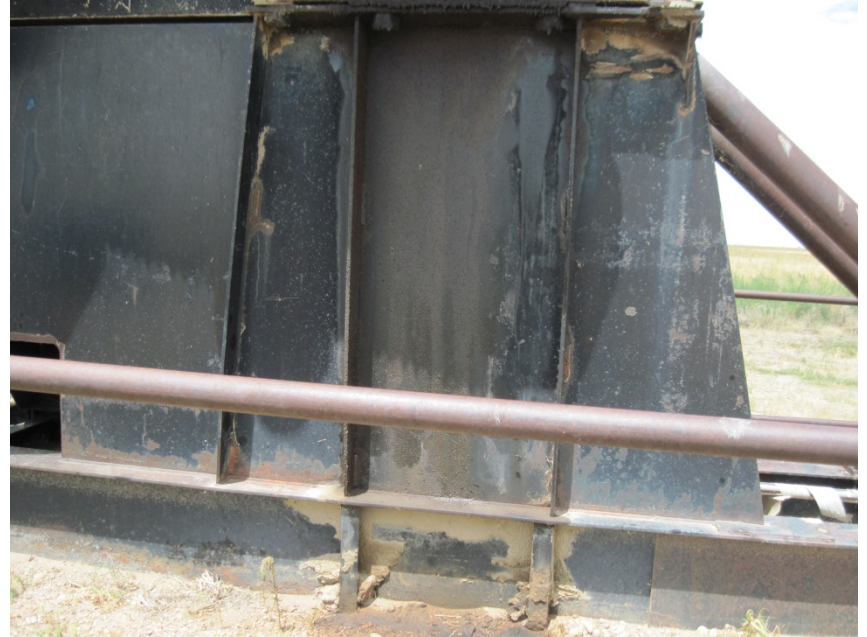
Stained soil from leaking gear box
