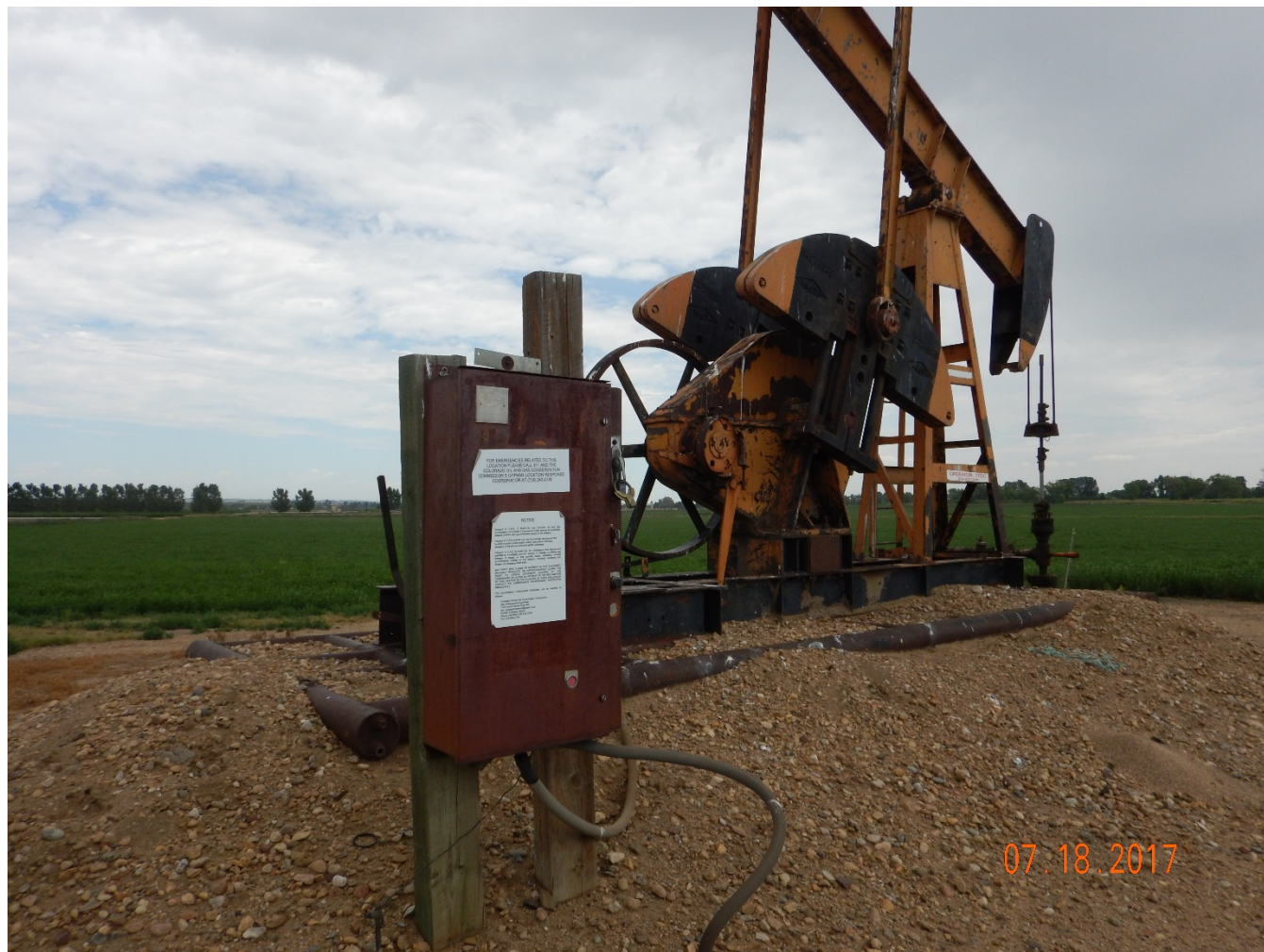
Figure 2 - COGCC emergency contact information affixed to electrical control panel.
