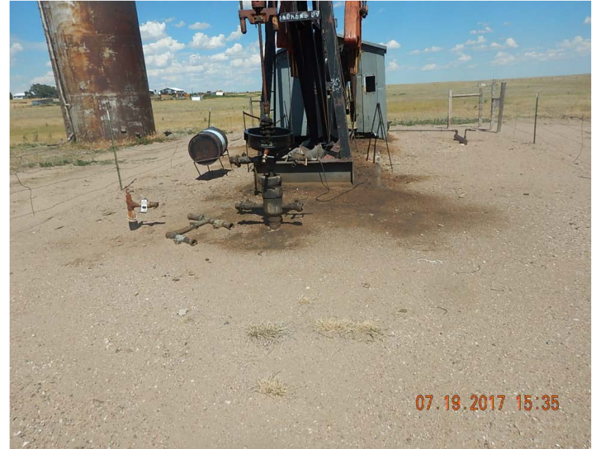
Photo 1: Stained soil at wellhead. TA well. Bradenhead not plumbed to surface.
