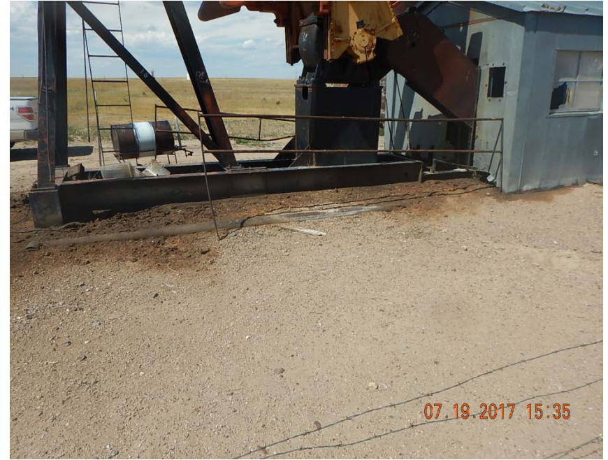
Photo 3: Stained soil at pump jack
