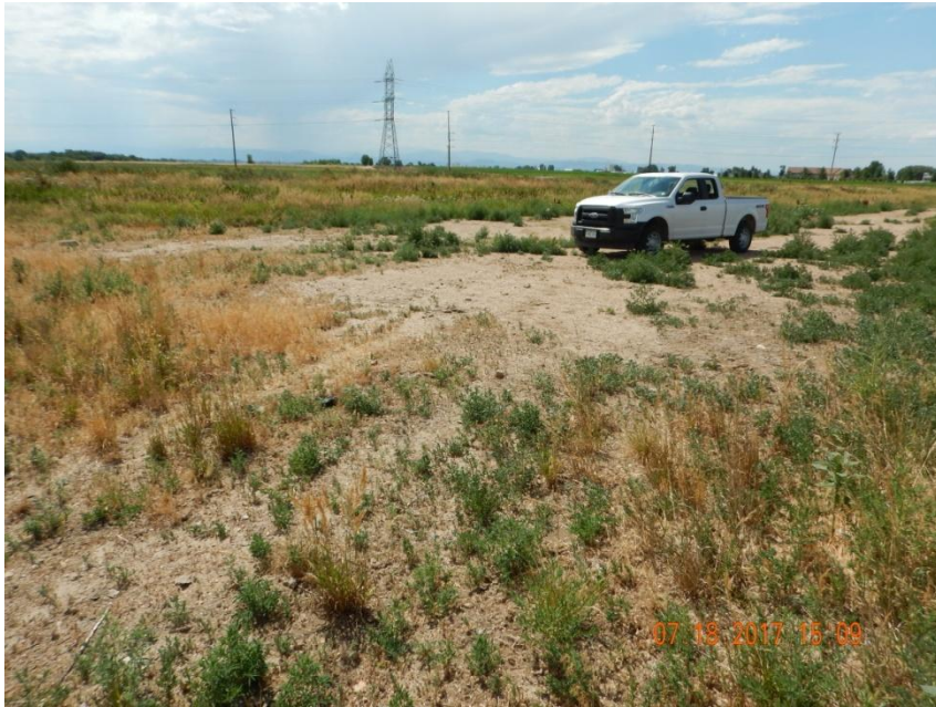
Photo 3. Photo taken from the battery location, facing West. Disturbance evident due to bare ground, gravel remains and weedy, annual vegetation not reflective of reference crop vegetative levels. The battery location has not been reclaimed per Rule 1004.
