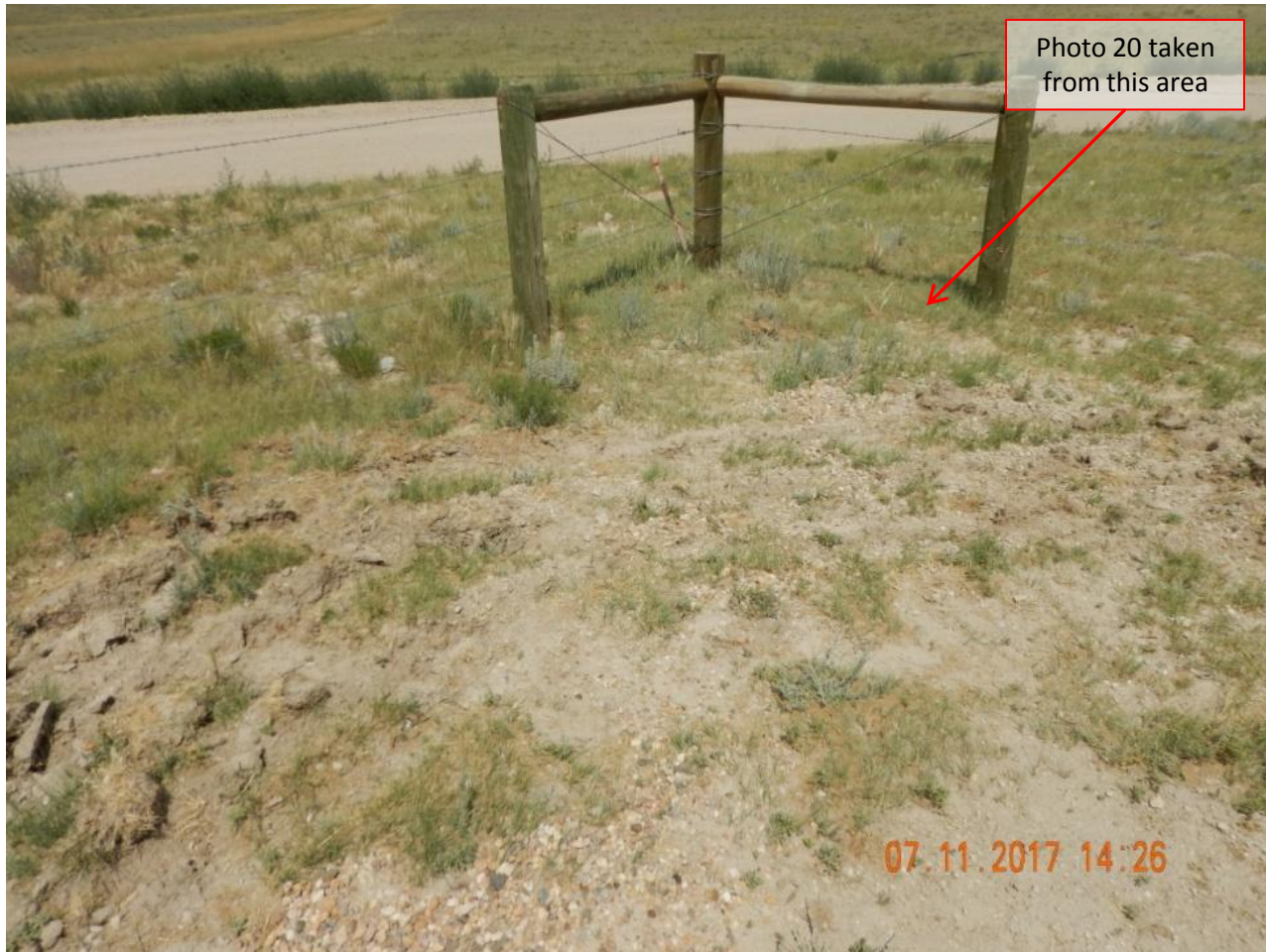
Photo 19. Photo taken just beyond the sediment trap, facing Northeast. Photo illustrates the surface roughening BMP is no longer in proper functioning condition, as it appears sediment discharge has filled in the BMP.
