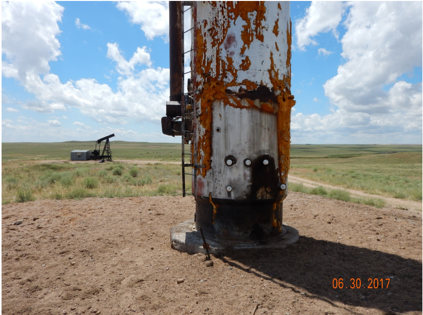
Figure 2 - Vertical heated separator remains on location.
