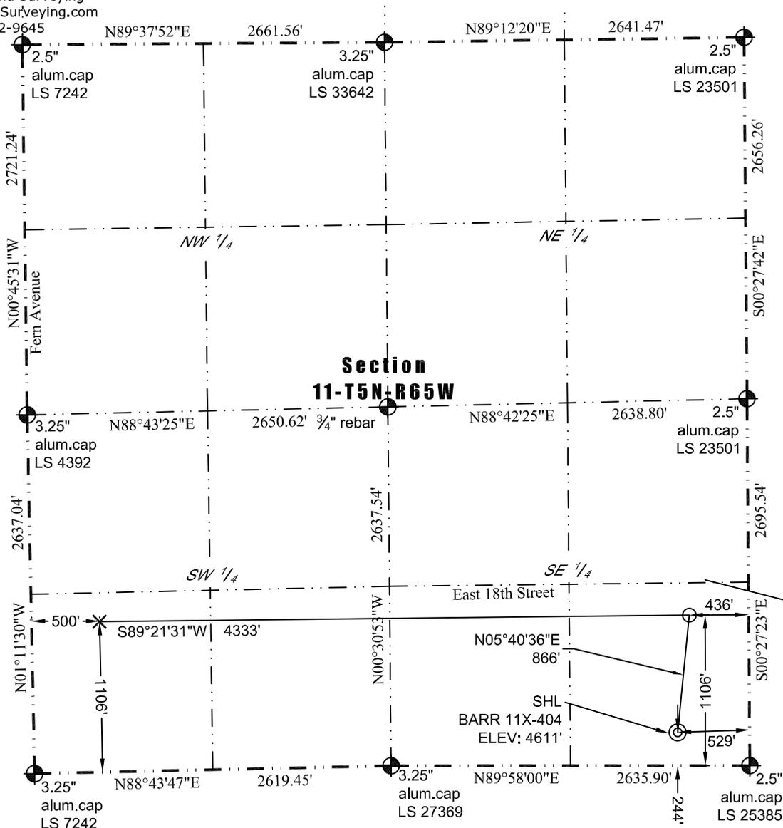
In accordance with a request from Barney Hammond of PDC Energy, Inc., Washburn Land Surveying, LLC has determined the location of the **BARR 11X-404** well site to be SHL: 244' FSL and 529' FEL, (BHL: 1106' FSL and 500' FWL), as measured at ninety (90) degrees from the section lines of Section 11, Township 5 North, Range 65 West of the 6th Principal Meridian, Weld County Colorado.
