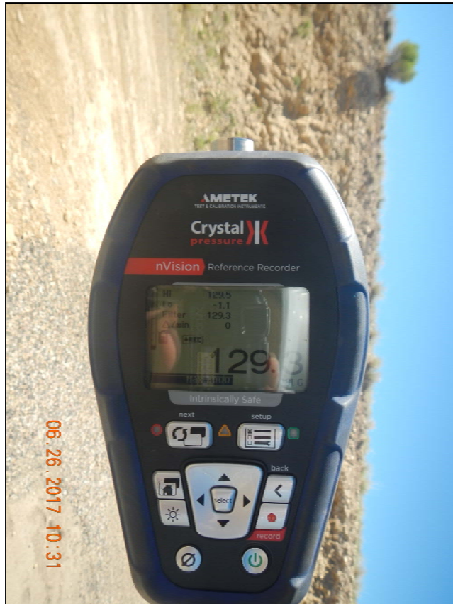
Photo 1. Gauge at beginning of test. 129.4 psi.
