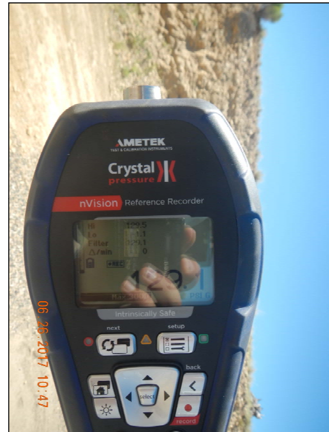
Photo 2. Gauge after 15 minute test. 129.1 psi.
