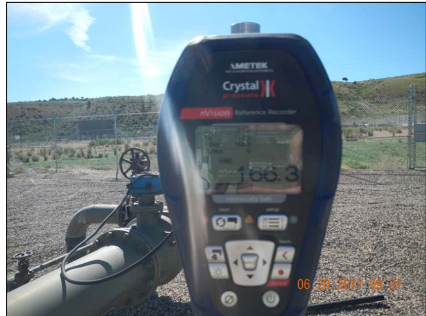
Photo 2. Gauge after 15 minute test. 166.3 psi.
