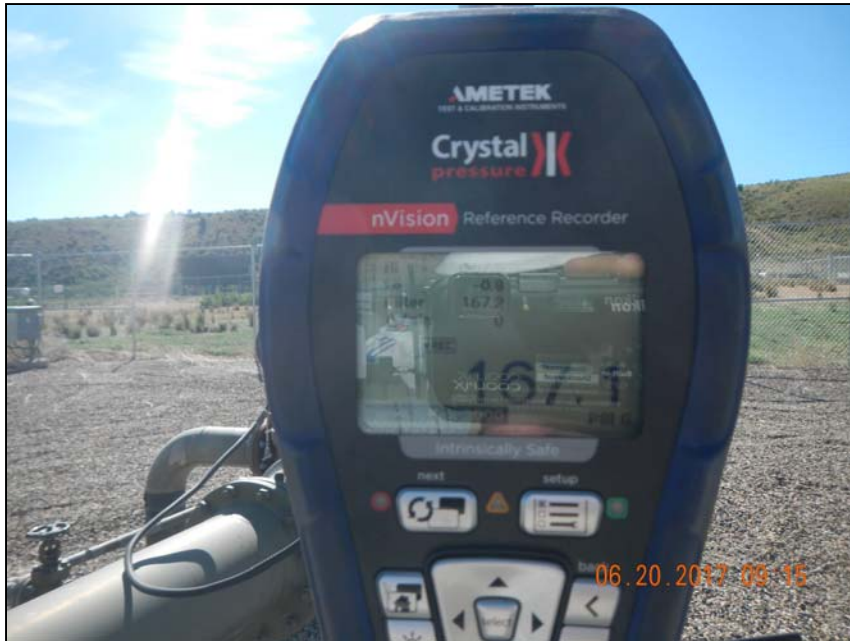
Photo 1. Gauge at beginning of test. 167.1 psi.
