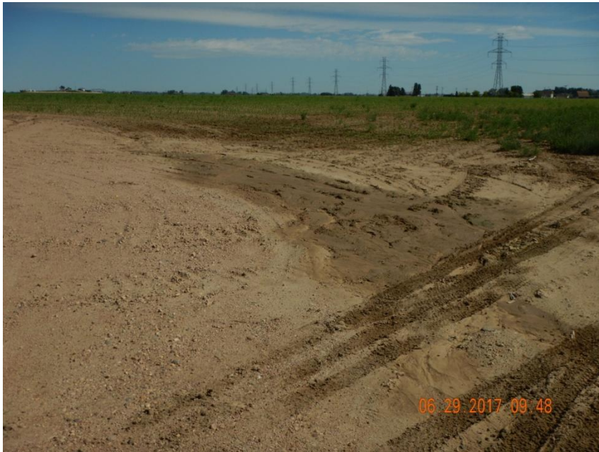
Photo 1. Photo taken from the northeast location, facing North. Appears stormwater and/or irrigation water run-on is flowing onto location which then travels across the eastern location through the wells. Gully erosion is occurring along the eastern location and off location.
