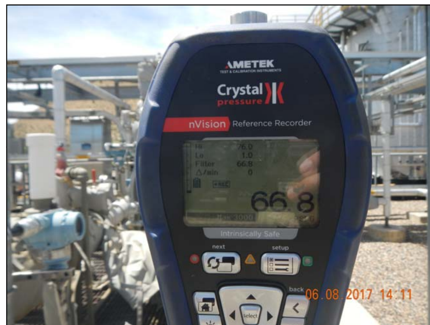
Photo 2. Gauge after 15 minute test. 66.8 psi.
