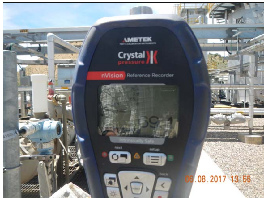
Photo 1. Gauge at beginning of test. 69.1 psi.
