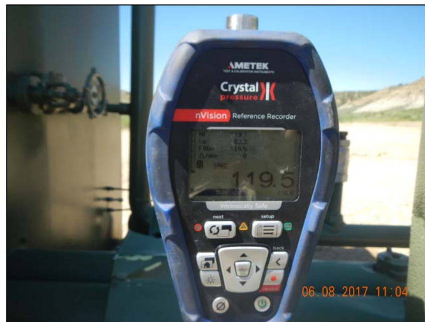
Photo 2. Gauge after 15 minute test. 119.5 psi.
