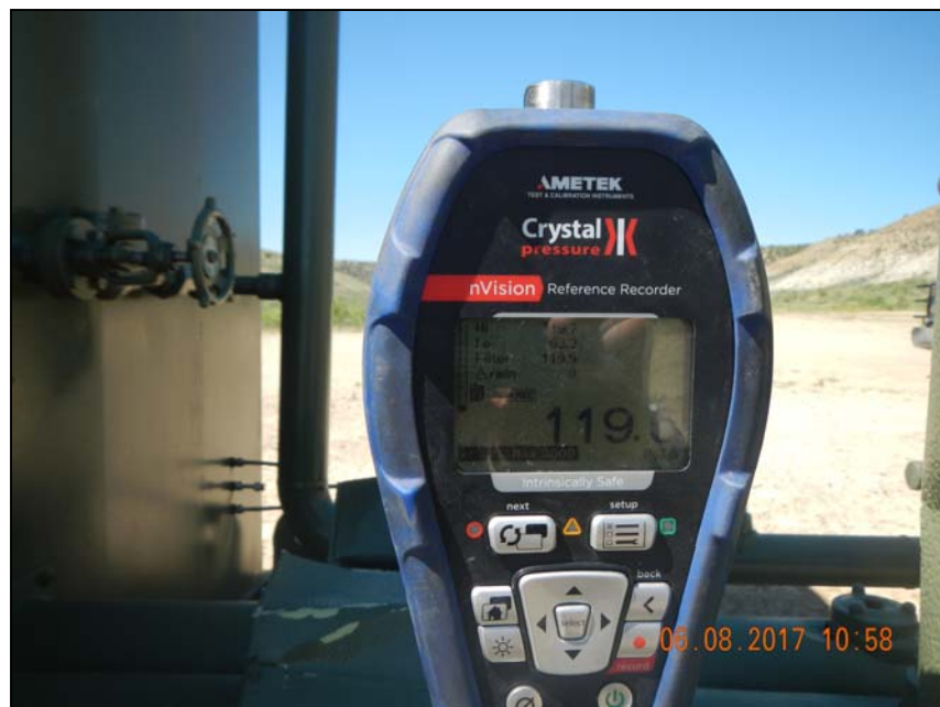
Photo 1. Gauge at beginning of test. 119.6 psi.
