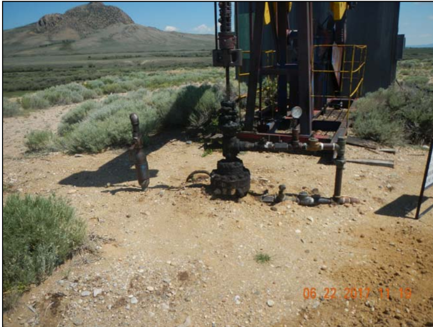
Photo 5. In use and not in use risers at wellhead.
