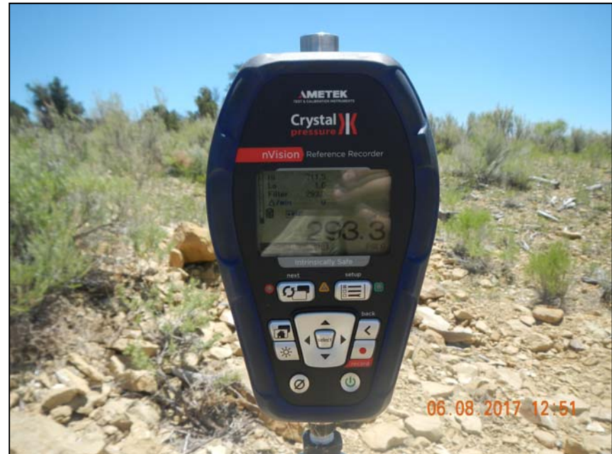
Photo 2. Gauge after 15 minute test. 293.3 psi.
