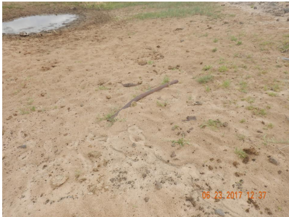
Photo 5: Photo of pipe debris found at the pit.
