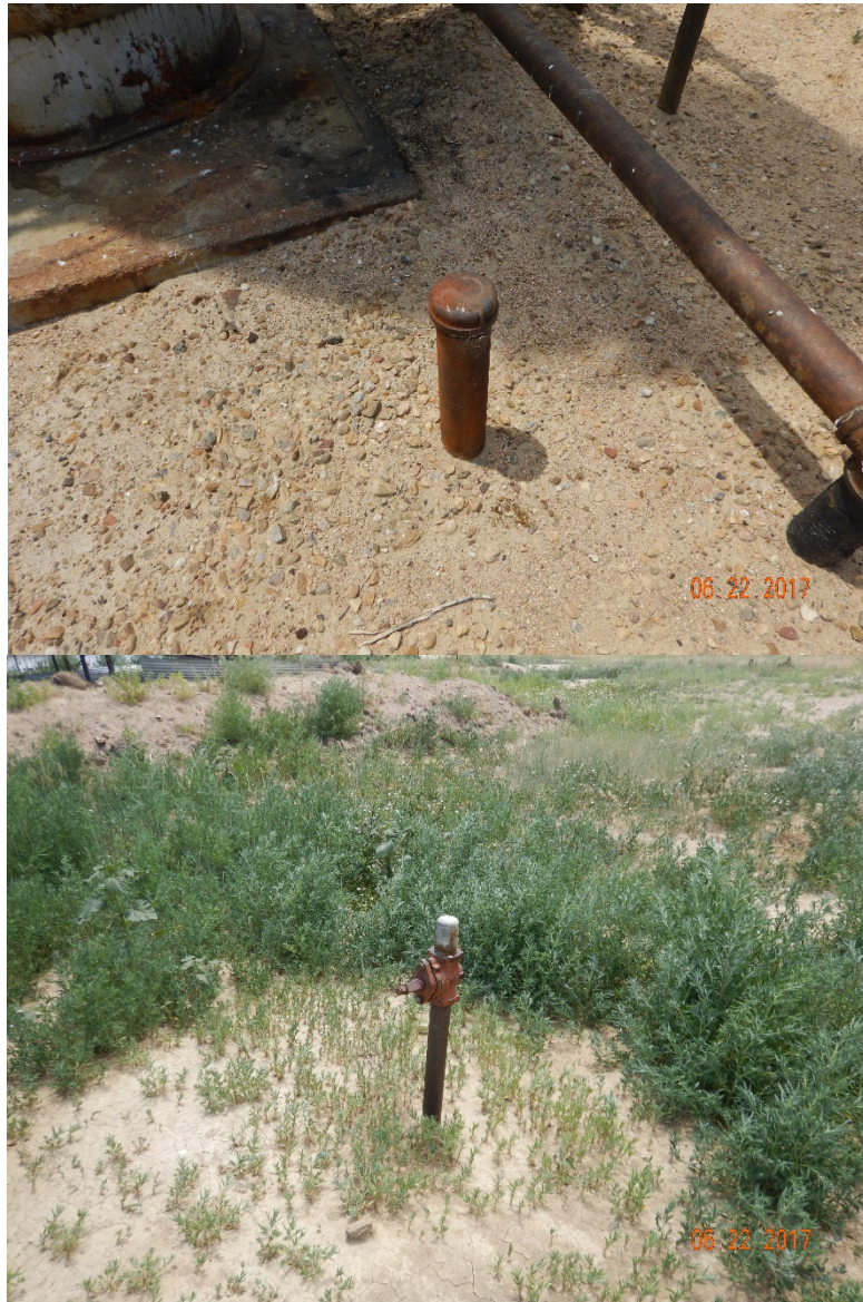
Figure 12 - Capped flowline risers located east and south of treater.
