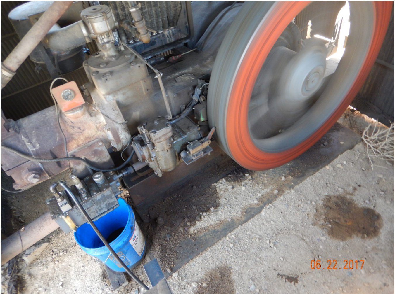
Figure 5 - Localized, oil-stained soil beneath prime mover (inside of shed).
